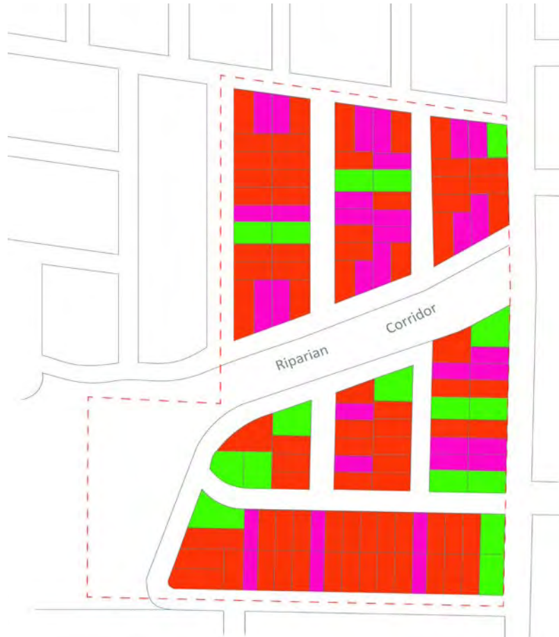
Figure 2.1 – Example subdivision illustrating a net lot density of 15 dwellings/ha using a mix of lot sizes
